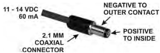
Figure 2. External Power Connector
